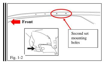
(b) Align the pins of the "RHF" (right hand front) side clamp/support (passenger side) to the second set of roof rail mounting holes from the front of vehicle (Fig. 1-2).
