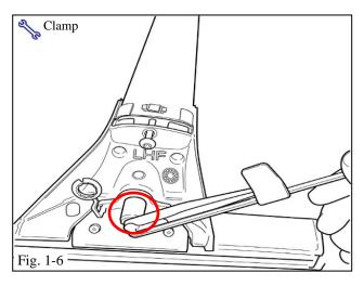
(d) While holding the clamp with the pins aligned into rail holes, use the supplied torque wrench, torque each main attaching screw to 9 N-m (71 in-lbs.) (Fig. 1-6).
