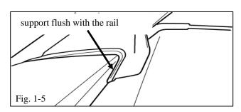
NOTE: Ensure the pins are in rails holes. Ensure pads located underneath the supports are flush to the rail for proper assembly (Fig.1-5).
