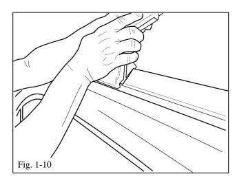
(h) Slide top of the cover around the bar and snap in the tabs at the base of the cover onto clamp/support (Fig 1-10).
