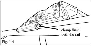
(c) Adjust by sliding the LHF side clamp/support (driver side) inward or outward to align clamp/support pins with the opposite roof rail mounting holes for snug fit (Fig. 1-3 &1-4).
